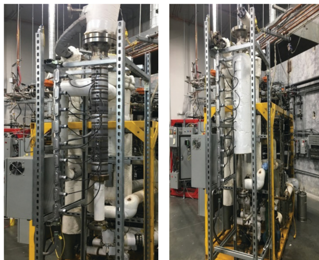
Fig. 2 Pilot-scale reactor with (left) and without (right) insulation, where band heaters are visible and wrapped around the reactor. The full piping and instrumentation diagram is available in Fig. S6 of the ESI.†
