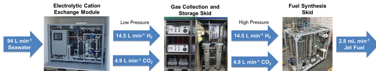
Fig. 13 NRL modular seawater-to-fuel system consisting of an electrolytic cation exchange module (E-CEM), gas collection and storage skid and fuel synthesis skid. The pilot-scale system can produce up to four liters of jet fuel per day ( 2.8 \text{ mL min}^{-1} ).
